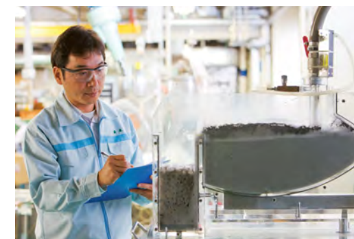
Deinking simulation using flotation deinking tester.
