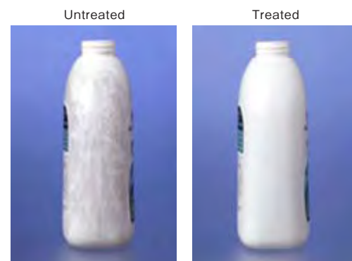
The effects of antistatic agents on plastic products (example of dirt chamber test results)
