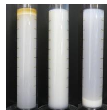
Emulsion Stability :Observe oil separation at top or bottom Measure oil layer
